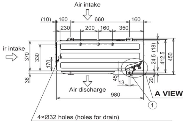
When using a drain pipe, install the drain socket (field supply) on to the drain hole. Seal the other drain hole with the rubber cap.
