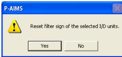
Clicking on the **Reset Filter sign** button in the upper right of the screen when an indoor unit is selected displays a confirmation message. Click on the **Yes** button to clear the filter sign. Click on the **No** button to cancel the reset.
