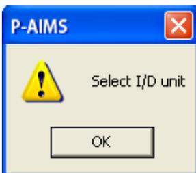
An error message is displayed if the user clicks on the **Reset Filter sign** button when no indoor unit is selected. Select the indoor unit before clicking on the **Reset Filter sign** button.
