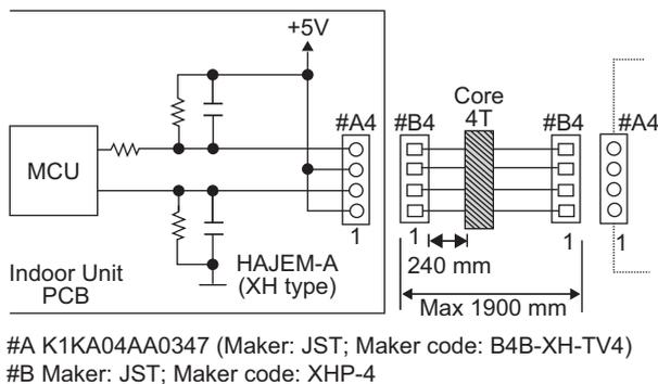
Note: The wire length from indoor unit to the external interface must be within 1.9 meters. The wire must be double insulation type and a ferrite core to be added to reduce noise. Proposed core spec is J0KE00000147 with Heat Shrinkage Tube.
