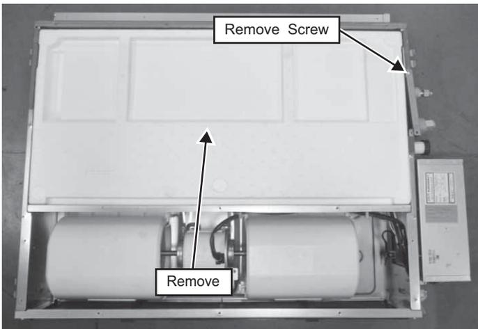
2 Unscrew 5 screws on the Evaporator and remove 2 sensor from holder and remove Evaporator from the unit.
