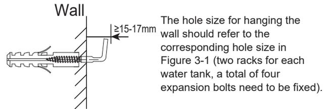
After the expansion bolt is tightened, the distance between the inner side of the bolt and the wall surface should be controlled within 15mm-17mm, as shown in the figure.
