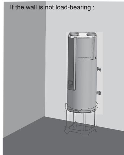
It is mandatory to install the water heater on a support. Place the water heater on the bracket to mark the fixing points. Make the holes and then reinstall the water heater in its place. The anti-tilting fixing by the upper bracket is obligatory (fixing Ø 10mm minimum adapted to the wall).
