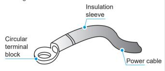
If it fails to crimp the insulated circular terminal block due to on-site limitations, connect the power cables of the same diameter to both sides of the power supply terminal block of the IDU, as shown in the figure below.
