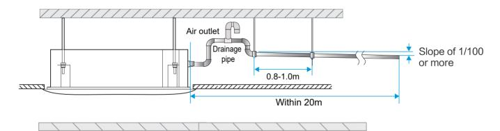
The end of the drainage pipe must be more than 50mm above the ground or from the base of the water discharge slot. In addition, do not submerge it in water. To discharge the condensed water directly into a ditch, the water discharge pipe must bend upwards to form a U-shaped water plug to stop odors from entering the room via the water discharge pipe.
