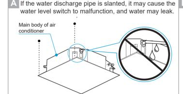
Adjust the position of the main body to ensure that the interval of the four sides of the ceiling is even, and the bottom surface of the main body should be recessed from the bottom surface of the ceiling by 10-12mm.
