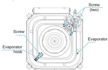
Remove the screws fixing the evaporator and the pump bracket in place, and remove the evaporator.
