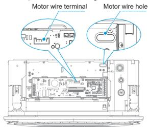
After removing the three bolts securing the motor in place, pull out the terminals according to the motor wire path. Remove the three motor bolts at the positions shown in the figure, pull out the terminals according to the motor wire path, and remove the motor.
