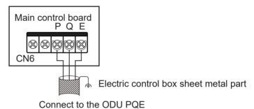
System: The maximum total length of the P/Q/E communication cable of the IDU and ODU can be up to1200m, and can be connected in serial, as shown in the figure below:
