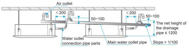
Drainage pipes from multiple units are connected to the main drainage pipe to be discharged through the sewage pipe.
