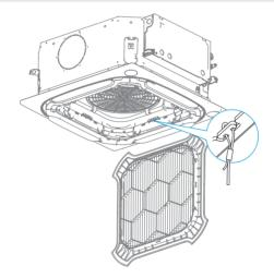
Install the suction grille back into the corresponding position, and push it up slightly at the grille clamp position to ensure that the grille buckle is fully engaged in the slot of the panel, and the grille is in the closed position.
