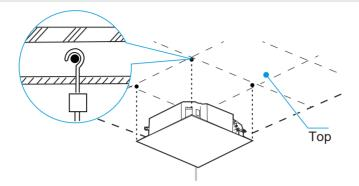
(3) Use the hex nuts on the four mounting hooks to adjust evenly and make sure the main body is level.
