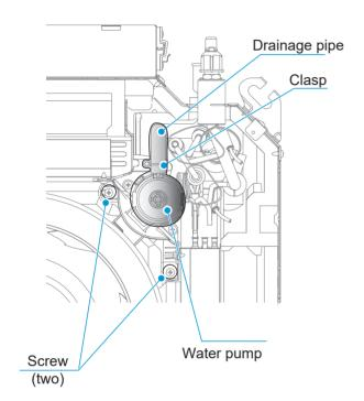
Remove the screws fixing the water pump and the pump bracket in place, and remove the water pump.
