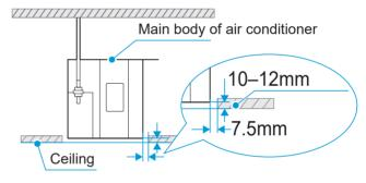
C After adjusting the main body position and level, tighten the nuts on the mounting hook to secure the air conditioner in place.
