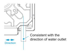
When connecting the drainage pipe, do not pull the drainage pipe forcefully, or it may become loose. The lateral pull-out of the drainage pipe should be within 20m, and a support point should be set every 0.8–1.0m to avoid air resistance caused by the deflection of the drainage pipe. The drainage pipe shall be equipped with a support point every 1.5-2.0m.
