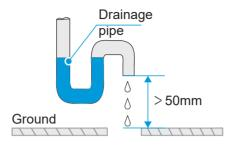
· Connection method of the drainage pipe:
