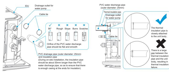
The drainage pipes of the unit (especially the indoor part) must be evenly wrapped with thermal insulation pipes and fastened with cable ties to prevent air from entering and producing condensate water.
