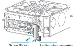
Screw (three) Sealing plate assembly
