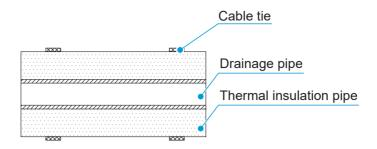
To prevent water from flowing back into the air conditioner when it stops running, the drainage pipe should be inclined downward to the outdoor side (drainage side), with a downward slope of 1/100 or more. The drainage pipe should be positioned in the same direction as the drainage outlet of the unit body in a left and right direction, so that the drainage pipe does not expand and collect water; otherwise, it may cause abnormal noise.
