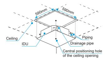
Confirm the installation hook position according to the installation hook holes located in the four corners of the mounting cardboard.
