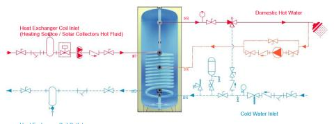
Heat Exchanger Coil Outlet (Heating Source / Solar Collectors Cooled Fluid)
