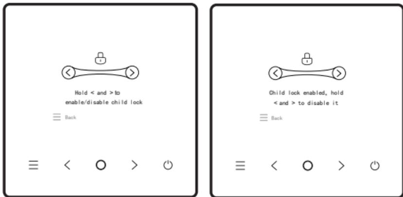
The child lock serves to prevent mis-operation of the device. After it is enabled, the buttons of the device will be locked and cannot be operated until the child lock is unlocked.
