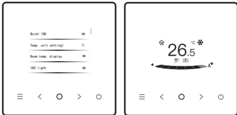
After the room temperature display is enabled, if you return to the home page and does not operate the device, the device will automatically display the room temperature and presents a room temperature icon.
