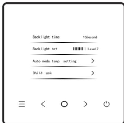
The backlight brightness has 10 levels, used to set the display brightness of the device. The brightness increases from level 1 to 10. You can press "○" to adjust the backlight brightness.
