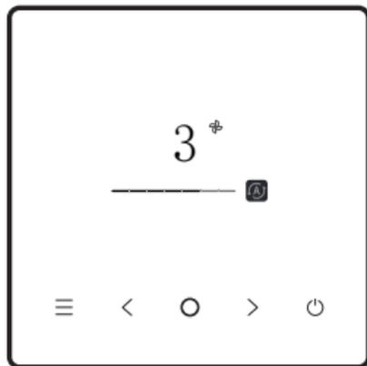
Select the fan speed on the menu, and press "○" for confirmation. After entering the fan speed interface, press "<" or ">" to select the operating speed, or press "≡" to return to the menu.
