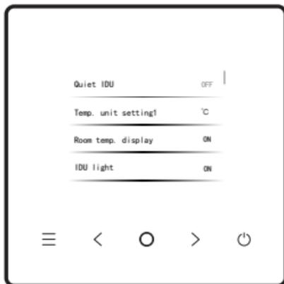
After "Quiet IDU" is enabled, the IDU will operate in silence.
