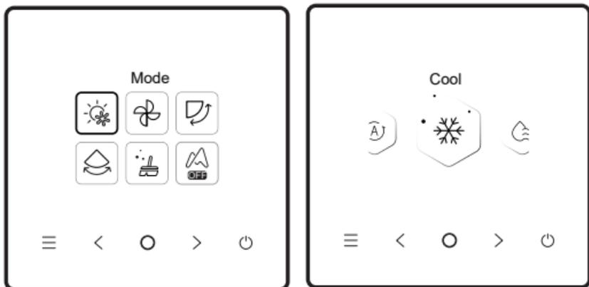
Select the mode on the menu and press "○" for confirmation. After entering the mode, press "<" or ">" to select the operating mode, and press "○" for confirmation. Or press "≡" to exit.
