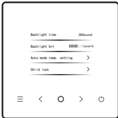
The backlight time can be set to 15s, 30s, or 60s. After the setting, if the device fails to receive any command within the set backlight time, it will enter the standby interface.
