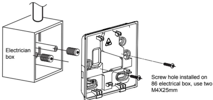
When installed on the wall:
