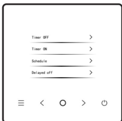
Select the timer function on the menu, and press "○" for confirmation. After entering the timer interface, press "<" or ">" to select the corresponding timer, and press "○" to start function setting.
