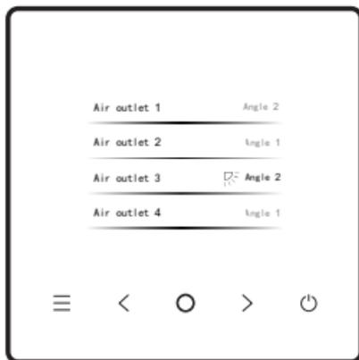
Select the swing up/down function on the menu, and press "○" for confirmation. After entering the swing interface, press "<" or ">" to select the air outlet to be controlled, or press "<" or ">" to adjust the swing angle.
