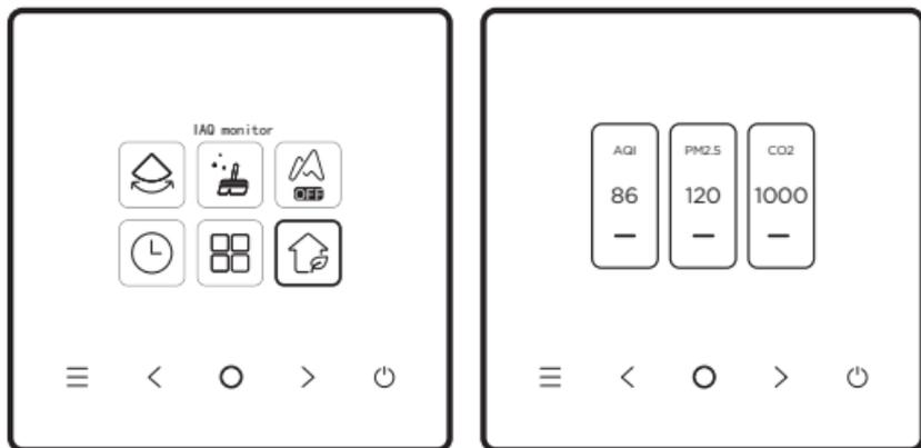
Select the IAQ function on the menu, and check the air quality indicators such as AQI, PM2.5 and CO2 in real time.
