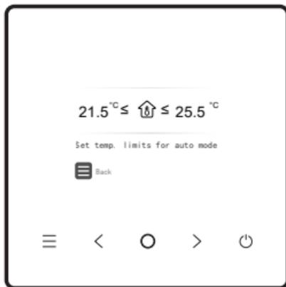
The temperature setting in auto mode enables you to set the temperature in auto cooling/heating mode, and maintain the indoor temperature within the set range.
