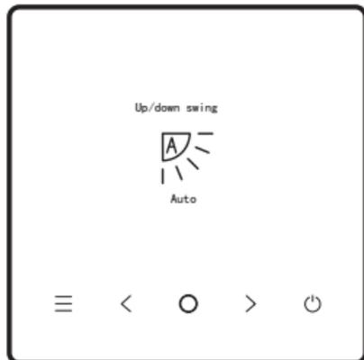
Select the swing (left/right) up/down function on the menu, and press "○" for confirmation. After entering the swing interface, press "<" or ">" to adjust the swing angle, or press "≡" to return to the menu.
