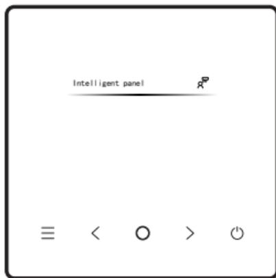
Select the setting on the menu, and press "○" for confirmation. After entering the function setting interface, press "<" or ">" to switch the function, and press "○" to enable the selected function.
