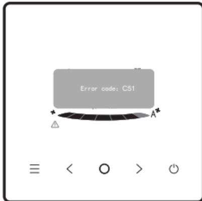
1. In case any IDU or ODU fails, the wired controller displays the fault code. In case a communication fault occurs between the wired controller and any of the IDUs, the wired controller reports "C51".
