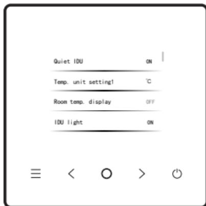
After the IDU light is enabled, the IDU display LED will light up. After the IDU light is disabled, the IDU display LED will turn off. You can press "○" to turn on or off the IDU light.
