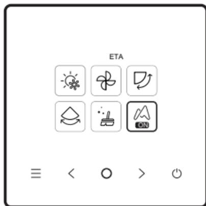
Select the ETA function on the menu, and press "○" to enable or disable the ETA function. The ETA function is real-time energy saving.
