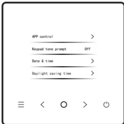
After "Keypad tone prompt" is enabled, the wired controller will operate in silence.
