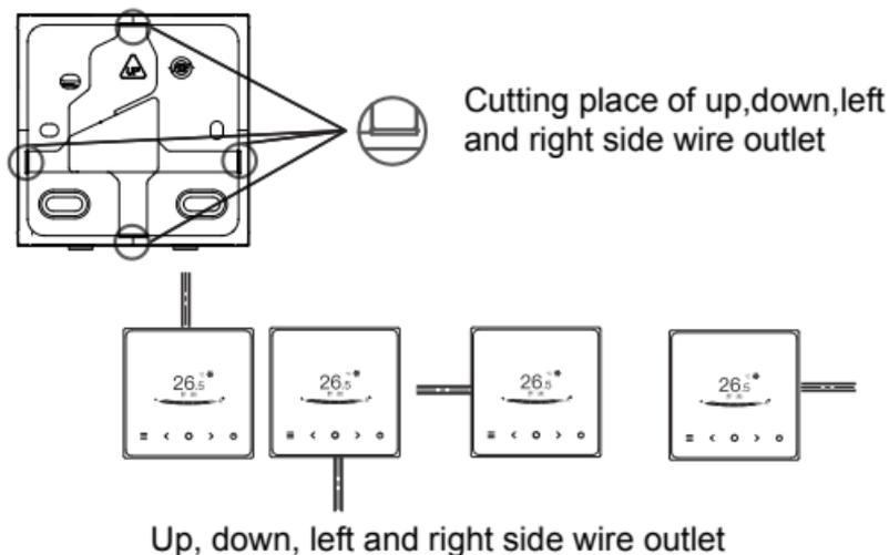
**Lead the 2-core shielded cable through the wiring hole in the bottom cap of the wired controller, and use screws to reliably fasten the shielded cable onto terminals X1 and X2. Then fix the bottom cap of the wired controller onto the electrical box by using pan head screws.**
