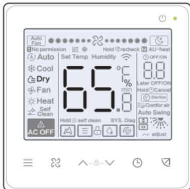
In dry mode, press " $\wedge$ " and " $\vee$ " to change humidity in the range of 35-75%.
