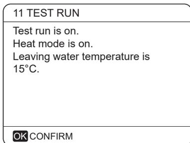
During HEAT MODE test running, the default target outlet water temperature is 35°C. The IBH (internal backup heater) will turn on after the compressor runs for 10 min. After the IBH runs for 3 minutes, the IBH will turn off, the heat pump will operate until the water temperature increase to a certain value or the next command is received.
