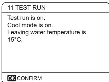
During COOL MODE test running, the default target outlet water temperature is 7°C. The unit will operate until the water temperature drops to a certain value or the next command is received.
