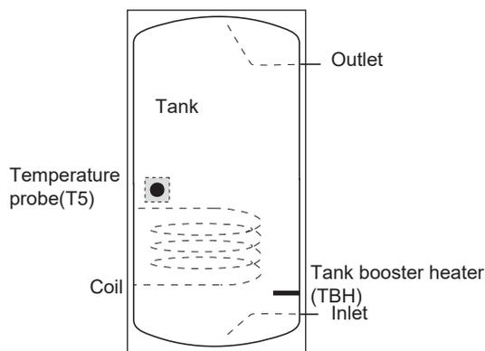
The booster heater should be installed below the temperature probe (T5).
