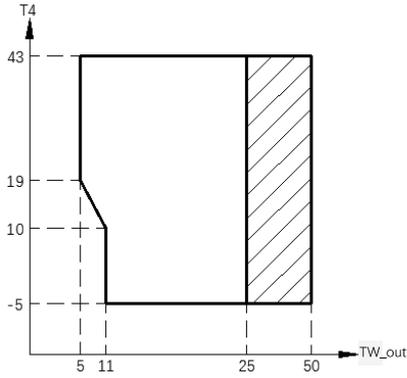
Operation range by heat pump with possible limitation and protection.
